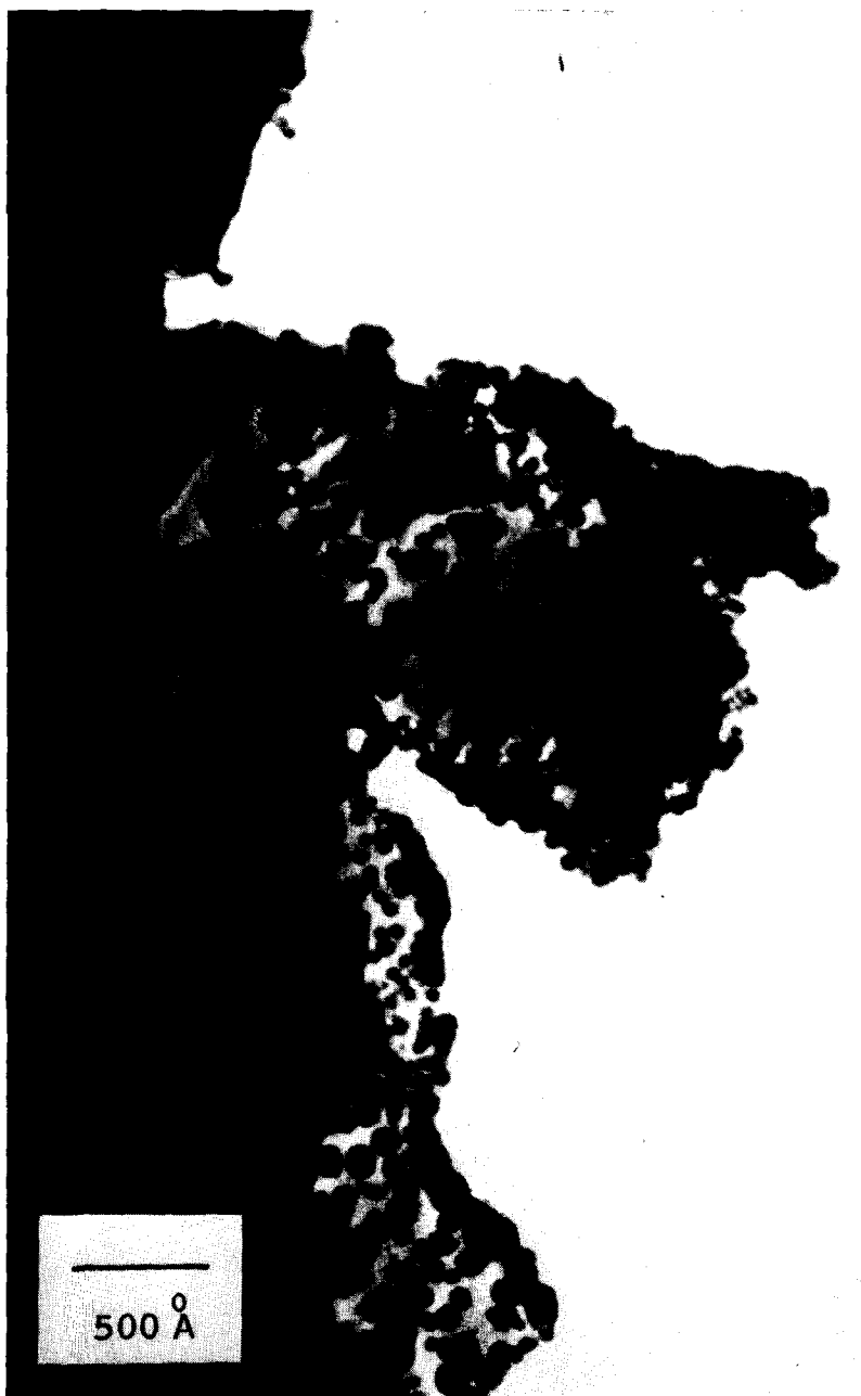
FIG. 2. Transmission electron micrograph of silver particles in the pore structure of Vycor quartz; \times 125,000 .
